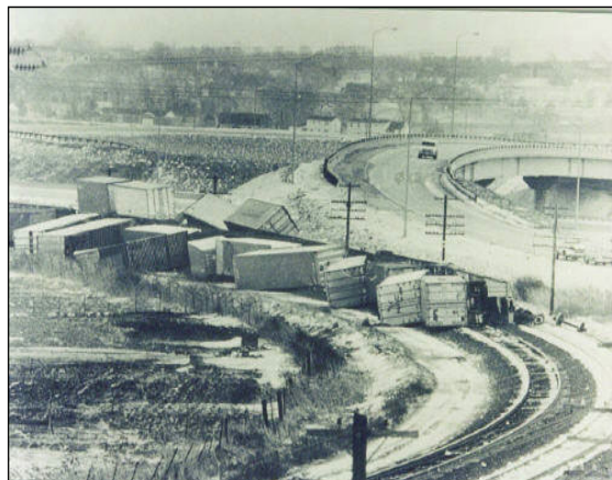
Wasatch Front, April 4-6, 1983 – 70 mph “East Winds” derailed this train in the Lagoon area. Peak gusts were recorded at 104 mph. (Source: Utah’s Weather and Climate , Photo: Ogden Standard Examiner )
